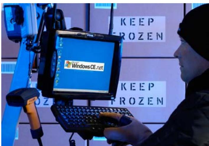
Handheld computers are available with long-range scanners, and can be used with powered vehicle-mount cradles. This makes them an intriguing option for forklifts in cold storage areas. However, handheld devices may not always be a viable option on forklifts, and the wireless or tethered handheld scanners that are typically used in conjunction with true vehicle-mount devices are
