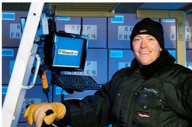
Standard data collection devices deliver less than substandard performance if they are consistently used inside freezers or exposed to frequent temperature changes. In fact, moving the computer between normal and cold areas is extraordinarily hard on just about every part of the device, even if it's ruggedised. In the short term, LCD screens fog up, batteries are unable to release enough energy,
